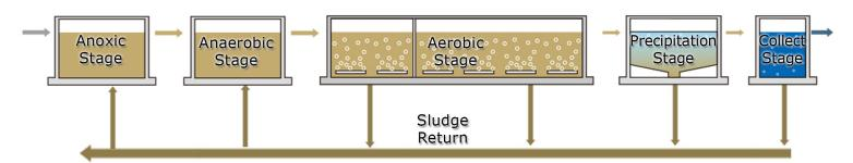
MBR-3C system wastewater treatment COD≤50mg/L, BOD5≤10mg/L, SS≈0mg/L
